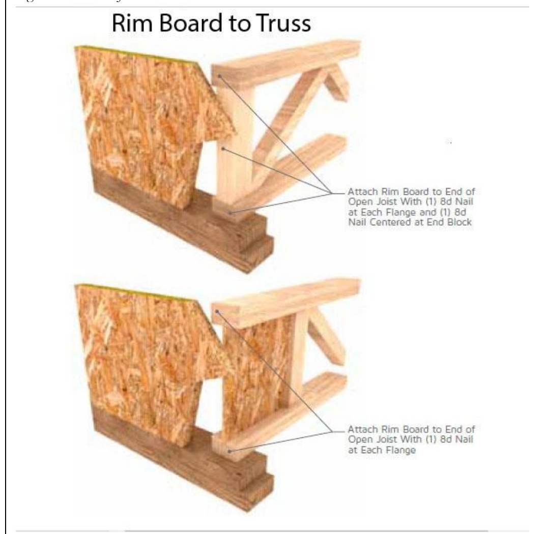
Figure 5.19 – Rim Joist
